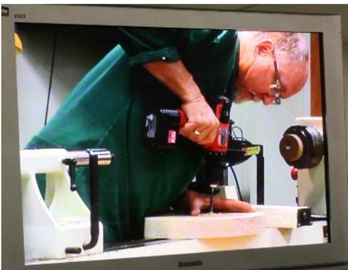
Keith drilling center and off-center holes for a screw chuck mounting (front side of platter)
