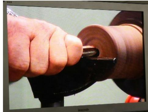
Keith Gotschall demonstrating "back hollowing" with a spindle gouge
