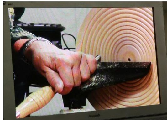
Cutting beads with a spindle gouge
