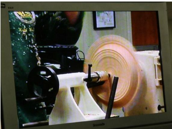
Keith turning backside of platter (mounted off-center on screw chuck)
