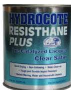
**Tip 2 -** For spraying this water-based lacquer from an airbrush or detail spray gun, cut with water to produce a 50-50 mixture. Spray until the surface just wets, but not puddles. Too much spray will produce a run or sag in the finish.
