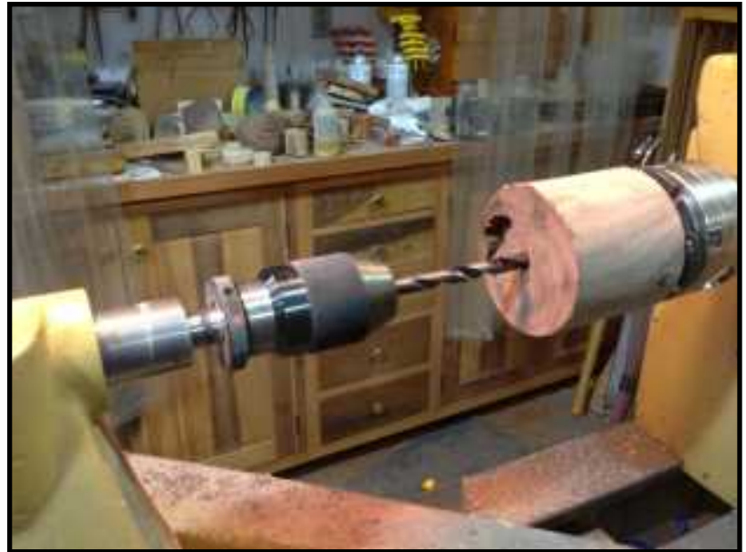
Fig 1. Typical On-Axis Drilling
