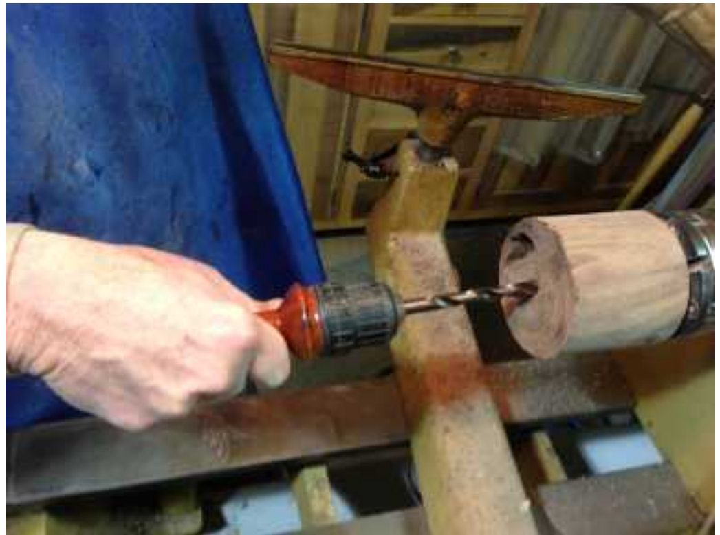
Fig 3. Handheld Bit Holder Drilling On-Axis Depth Hole
