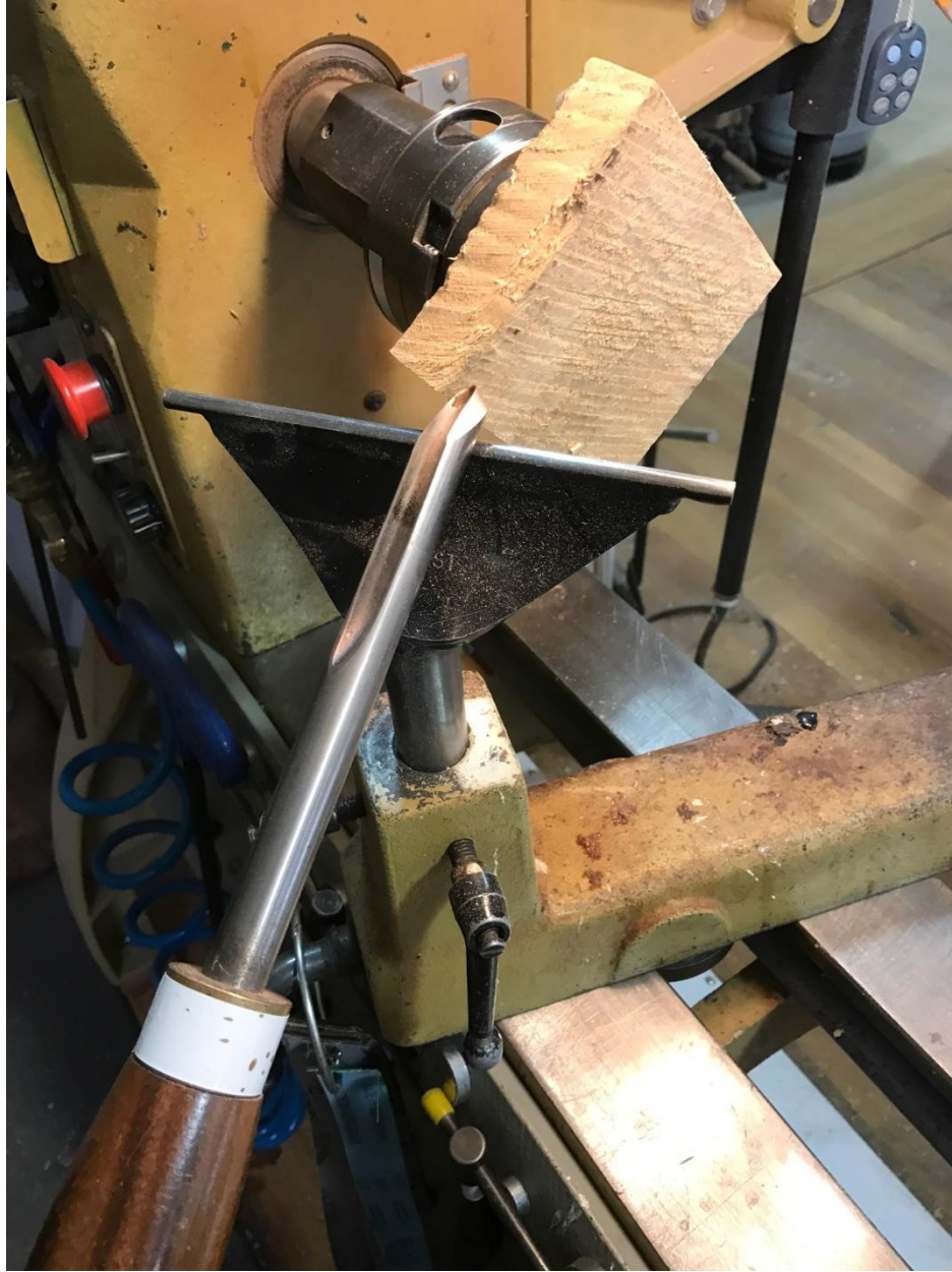
Fig. 2 “3-45” Pull Cut with Tool Rest at 45 degrees to Lathe, Tool Handle down at 45 degrees, Flute closed to 45 degrees
